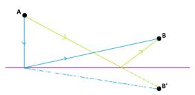
The shortest path from A to B' is the straight-line path.
