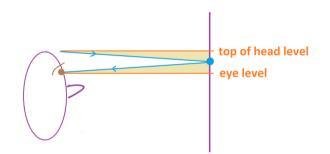
Because rays of light bounce off mirrors to keep angles the same, we see that the two triangles I've shaded are identical in all ways: angles, lengths, shape, and size. (One is just an upside-down version of the other.) This means that that the ray of light is bouncing off the point on the mirror halfway between the top-of-your-head level and eye level. This is where you put a piece of tape.
