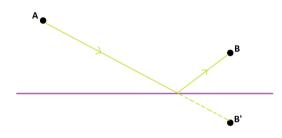
This must then give the shortest path from A to the wall to the point B.
